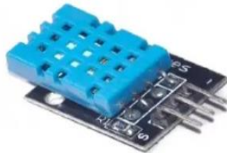
Figure 6: Actual image of DHT11 sensor [11]
