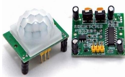
Figure 5: HC-SR501 PIR Sensor
